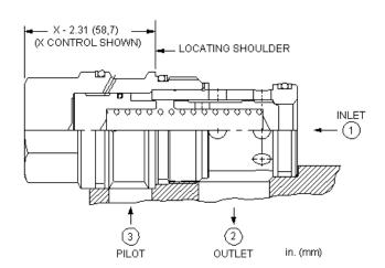
This valve is a spring biased closed, pilot-to-close check cartridge that has a 1.8:1 pilot ratio. The valve allows flow from port 1 to port 2 and blocks reverse flow. Pressure at the pilot port opposes pressure at port 1 at a ratio of 1.8:1. This valve is most often used in regeneration circuits.
