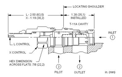
This valve is a spring biased closed, pilot-to-close check cartridge that has a 1.8:1 pilot ratio. The valve allows flow from port 1 to port 2 and blocks reverse flow. Pressure at the pilot port opposes pressure at port 1 at a ratio of 1.8:1. This valve is most often used in regeneration circuits.
