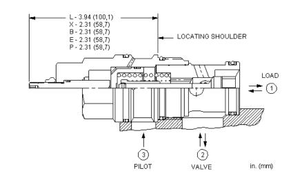
This valve is a pilot to open check valve. It has a non-sealed pilot, a steel seat, and is non-vented. It allows free flow from the valve (port 2) to the load (port 1) and blocks flow in the opposite direction. Pressure at the pilot (port 3) will open the valve from port 1 to port 2. Pilot pressure needed at port 3 to open the valve is directly proportional to the load pressure at port 1. Pressure at port 2 directly opposes pilot pressure.
