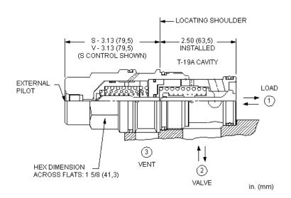
This valve is a pilot to open check valve. It has a sealed pilot, a steel seat, and is vented. It allows free flow from the valve (port 2) to the load (port 1) and blocks flow in the opposite direction. Pressure at the external pilot port will open the valve from port 1 to port 2. Pilot pressure needed to open the valve is directly proportional to the load pressure at port 1. The valve is insensitive to pressure at port 2 because the spring chamber references the vent (port 3).
