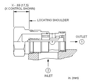
Free-flow, side-to-nose check valves are on/off circuit components that allow free flow from the inlet (port 2) to the outlet (port 1) and block flow in the opposite direction.
