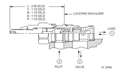
This valve is a pilot to open check valve. It has a non-sealed pilot, a steel seat, and is non-vented. It allows free flow from the valve (port 2) to the load (port 1) and blocks flow in the opposite direction. Pressure at the pilot (port 3) will open the valve from port 1 to port 2. Pilot pressure needed at port 3 to open the valve is directly proportional to the load pressure at port 1. Pressure at port 2 directly opposes pilot pressure.
