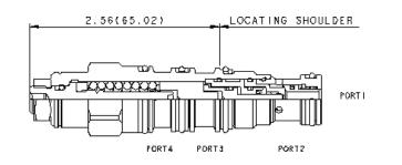
Vented counterbalance valves with pilot assist are meant to control an overrunning load. The check valve allows free flow from the directional valve (port 2) to the load (port 1) while a direct-acting, pilot-assisted relief valve controls flow from port 1 to port 2. Pilot assist at port 3 lowers the effective setting of the relief valve at a rate determined by the pilot ratio. Backpressure at port 2 does not affect the valve setting because the spring chamber references the vent (port 4).
