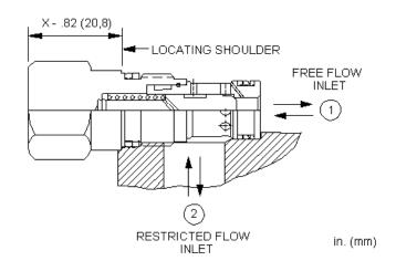
Free-flow, nose-to-side check valves with a bypass orifice allow free flow from port 1 to port 2. A customer specified orifice is included to restrict flow from port 2 to port 1. See technical data below for orifice range.
