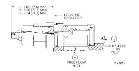
Needle valves with reverse-flow check are fully adjustable orifices used to regulate flow. They are infinitely adjustable from fully closed up to the maximum orifice diameter. An integral high-capacity check valve provides unrestricted flow from port 2 to port 1. They are not pressure-compensated.
