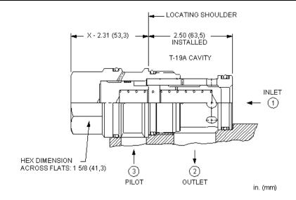
This valve is a spring biased closed, pilot-to-close check cartridge that has a 1.8:1 pilot ratio. The valve allows flow from port 1 to port 2 and blocks reverse flow. Pressure at the pilot port opposes pressure at port 1 at a ratio of 1.8:1. This valve is most often used in regeneration circuits.
