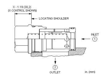
Free-flow, nose-to-side check valves are on/off circuit components that allow free flow from the inlet (port 1) to the outlet (port 2) and block flow in the opposite direction.
