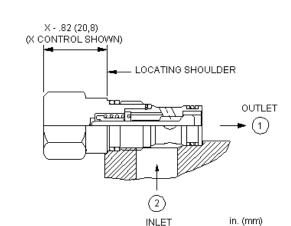
Free-flow, side-to-nose check valves are on/off circuit components that allow free flow from the inlet (port 2) to the outlet (port 1) and block flow in the opposite direction.
