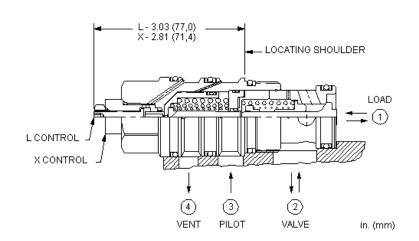
This valve is a pilot to open check valve. It has a sealed pilot, a steel seat, and is vented. It allows free flow from the valve (port 2) to the load (port 1) and blocks flow in the opposite direction. Pressure at the pilot (port 3) will open the valve from port 1 to port 2. Pilot pressure needed to open the valve is directly proportional to the load pressure at port 1. The valve is insensitive to pressure at port 2 because the spring chamber is referenced to the vent (port 4).
