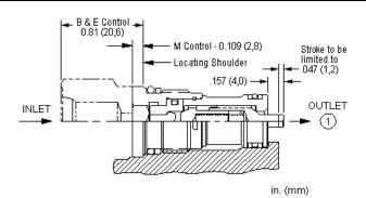
The phaser check is a pair of checks, back-to-back, with the poppet at port 1 mechanically actuated. The valve is meant to be installed into the piston of a cylinder. When the cylinder reaches the end of its stroke the poppet in the phaser check is shoved off its seat allowing flow through the piston. This allows two cylinders to get back into phase.
