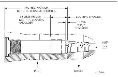
The single ball shuttle connects the higher of two work ports to the signal or common port. The signal is sensed at port 2.
