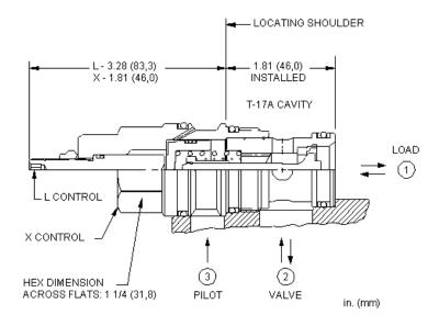
This valve is a pilot to open check valve. It has a sealed pilot, a Delrin seat, and is non-vented. It allows free flow from the valve (port 2) to the load (port 1) and blocks flow in the opposite direction. Pressure at the pilot (port 3) will open the valve from port 1 to port 2. Pilot pressure needed at port 3 to open the valve is directly proportional to the load pressure at port 1. Pressure at port 2 directly opposes pilot pressure.
