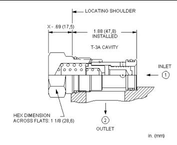
This valve was designed to be used in a parts-in-body, hot oil shuttle assembly. 2 valves, nose to nose, with a pin in between created the low side shuttle.
