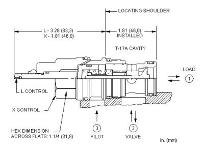
This valve is a pilot to open check valve. It has a non-sealed pilot, a Delrin seat, and is non-vented. It allows free flow from the valve (port 2) to the load (port 1) and blocks flow in the opposite direction. Pressure at the pilot (port 3) will open the valve, allowing flow from port 1 to port 2. Pilot pressure needed at port 3 to open the valve is directly proportional to the load pressure at port 1. Pressure at port 2 directly opposes pilot pressure.
